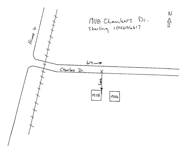
Work willbegin et (x) 614 East of Hiway 6 on the south side of Chambers Dr. At this point we will sore south out of the Row 65' to the meter location on the east side of the house.
