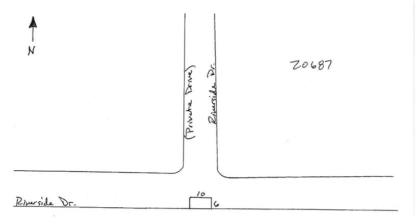
Work will be <u>Trenched</u> only on the south side of Riverside Drive in the intersection of Private Drive and Riverside. We will cut a 6×10' hole in the asphalt.
