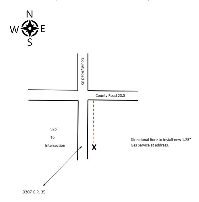
Work will begin at a point (X) 925 feet South of the intersection of County Road 20.5 and County Road 35, on the East side of County Road 35. At this point we will bore under County Road 35, in a Westerly direction.
